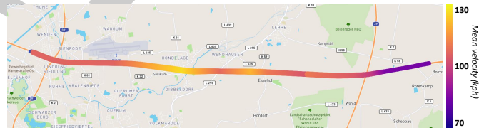
(a) Visualization of the vehicle perspective. The mean velocity measured by the loop detectors is displayed along the course of the road.
