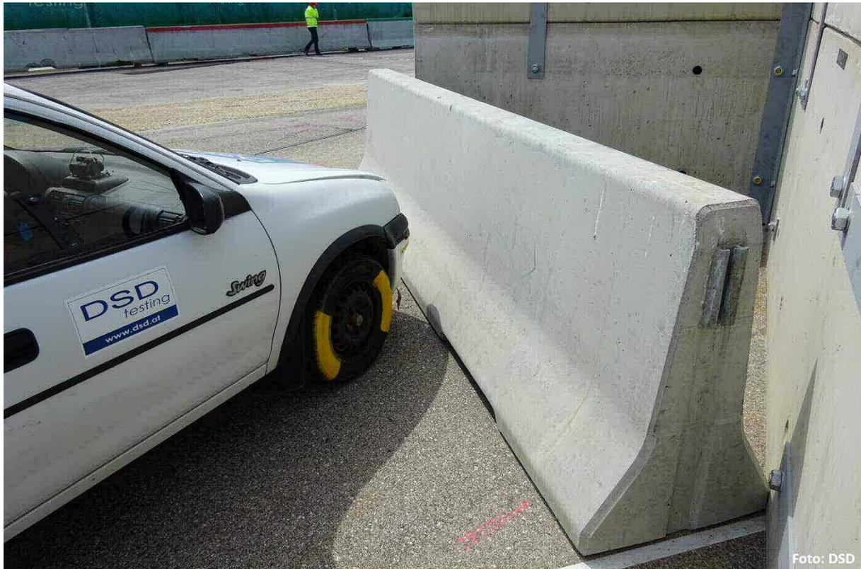
Abbildung 6: Anprallsituation Detail "BMV17001"
