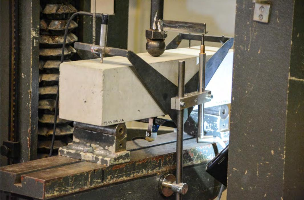
Splitting test illustration – specimen PC2.0\_T074\_1B before testing
