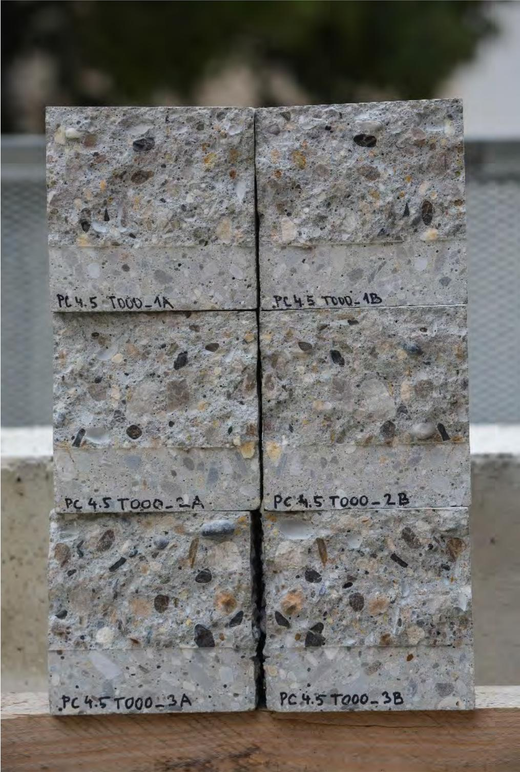
Specimens after fracture test – PC4.5\_T074
