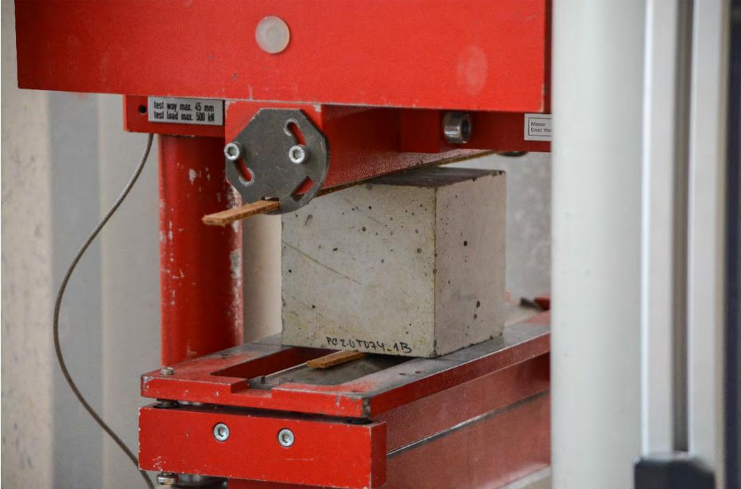
Splitting test illustration – specimen PC2.0\_T074\_1B after testing
