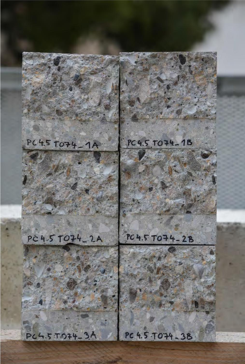
Specimens after fracture test – PC4.5\_T074\_2
