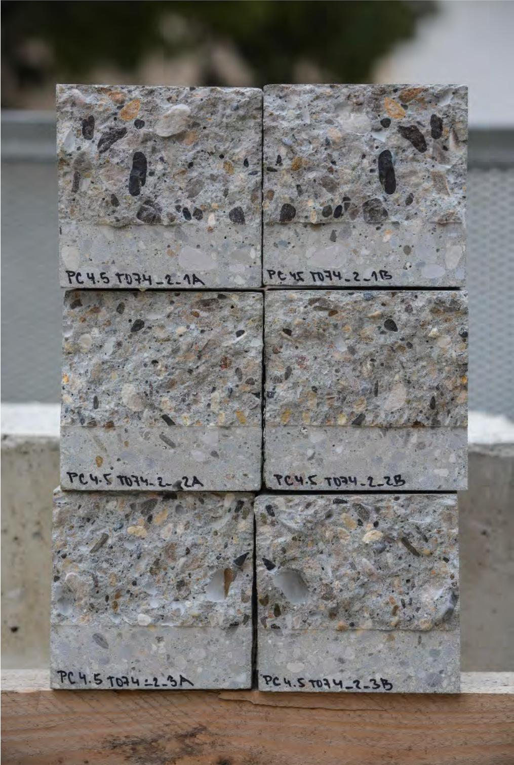
Specimens after fracture test – PC4.5\_T168
